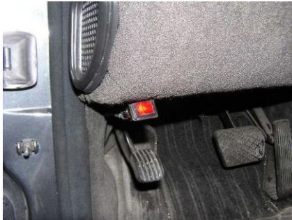
System Power Switch
